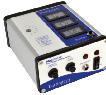
(b) Power supply and display unit
